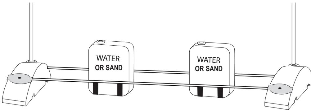
**Horizon is suitable for indoor or outdoor use. However if used in strong winds extra weighting may be necessary. Attach straps (not included) to the base poles to hold additional weights (not included).**
